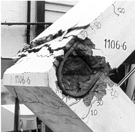
Figure 2.11 Spalling of side concrete cover in frame corner ( Type 3 ) when using spliced reinforcement loops. Photos from Johansson (1996) and Grassl (1999), respectively.
