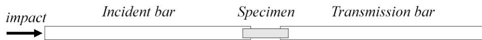
Figure 3.2 Illustration of a Split Hopkinson Tension Bar design, based on Wu et al. (2005)
